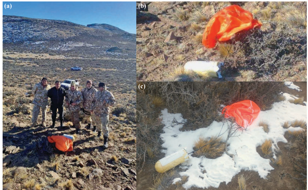
Figure 7. Landing sites of the DRS capsules in Argentina. (a) General terrain and the Search and Rescue team from the Governor’s Office of Santa Cruz Province. The bright orange parachutes of DRS1 (b) and DRS2 (c) were visible from distance. The white foam shell and release crown are finally also visible; the foam helped to insulate and waterproof DRS2 when it landed on snow.
